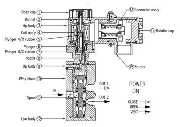
As signal pressure is being supplied, plunger (⑥) rises and creates a gap between the nozzle (⑨) and plunger (⑥) which results primary air pressure to push down the spool (⑪) and exhausts air to OUT2 (C2). When signal pressure has been turned off, the plunger (⑥) moves downward and blocks the channel. At the same time, air pressure pushes spool (⑪) upward and exhausts air to OUT1 (C1).
