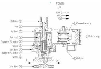
As signal pressure is being supplied, the plunger (6) rises and creates secondary a gap between the nozzle (9) and plunger (6) which results primary air pressure exhaustion. When signal pressure has been turned off, the plunger (6) moves downward and blocks the channel. At the same time, the air pressure will exhaust through the channel between the plunger (6), vent (2), and body cap (1).
